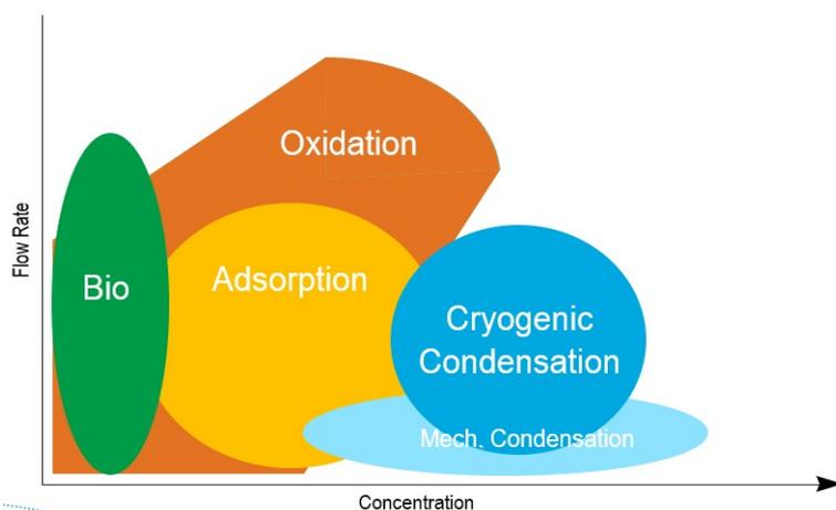
Figure 1: Alternative types of technology for solvent abatement and VOC recovery
