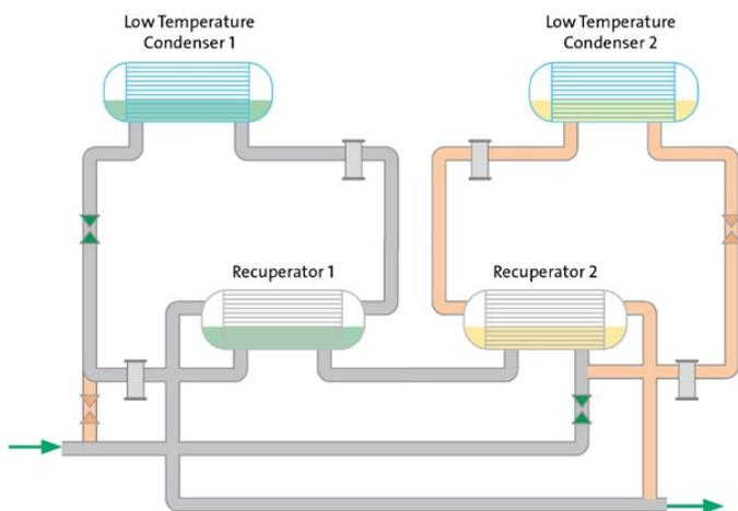
*Figure 2: Schematic of a Cryo-Condap® installation at a biopharmaceutical manufacturing site with recuperators used to pre-cool the incoming waste gas stream.*
